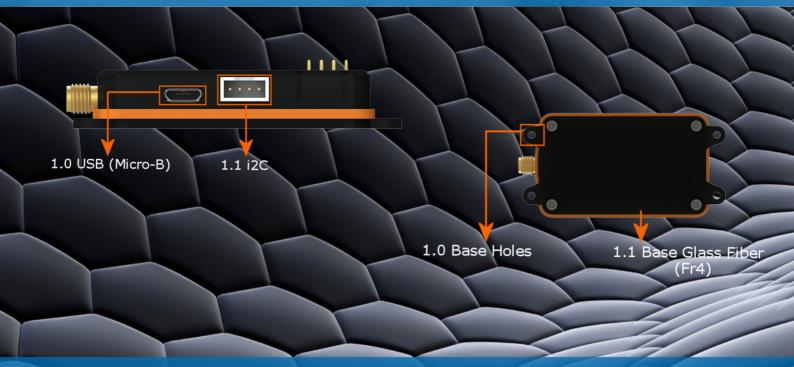
1.0- USB (Micro-B): Update and configuration RX.1.1- i2C: To connect future devices, OLED displays, IMU, etc.
