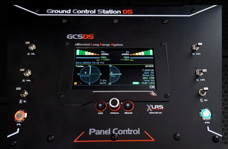
In the center of the GCSD5 there is a TFT IPS color screen with 4.3" high resolution that shows the current status of the GCS at all times, battery level, alarm messages, etc.
