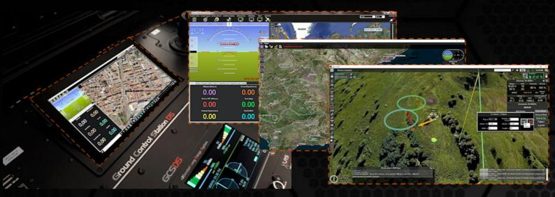
From the PC you can use any mapping software, that supports the Mavlink telemetry protocol, such as Mission Planner, QGroundControl, uGCS or similar, to be able to plot routes, establish waypoints and program specific tasks for your vehicle if you use an compatible autopilot (Cube, Pixhawk, APM or similar).
