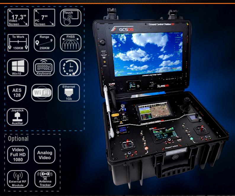
Ground Control Station for Radio Control, Mavlink Telemetry / Transparent Data Link, Video, Maps and Navigation for all types of applications with Aerial, Land or Maritime Vehicles
