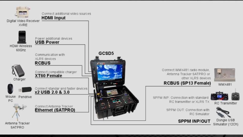
Radio Control: The GCS has an SPPM signal to send up to 16 RC channels, which allows you to assign various objects (Joysticks, Buttons, Switches, etc.) of the GCS to different RC channels and these will be sent to your RC system.
