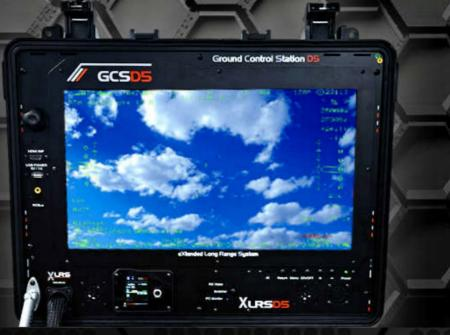
IPS LED video screen 17,3" Full HD 1920 x 1080 @60Hz, high brightness with 600-1000 nits and 1000:1 high contrast and 178° viewing angle.
