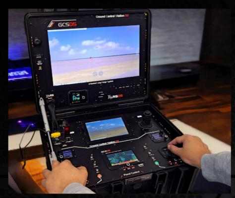
Connect the USB dongle of your RC simulator to the SPPM input of the GCSD5 to control up to 16 RC channels and simulate their operations with the GCSD5 controls.
