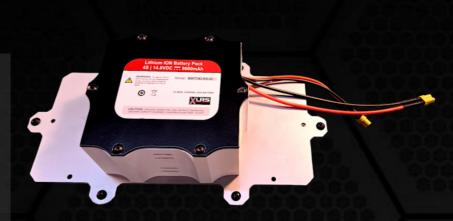
It incorporates a 4S/14.8V/9600mAh Li-ion battery, which has a protection circuit to prevent over-consumption, low and high voltage, temperature, as well as charging current control.
