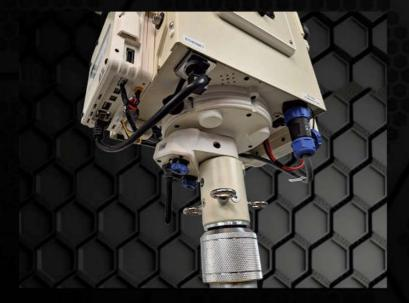
Ethenet - Wifi: SATPRO has a UDP server to which you can send received Mavlink telemetry packets and it will position itself automatically, you can also send commands to position SATPRO directly.
