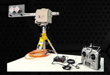
Optionally, a standard RC transmitter can be connected using the BTSD1V3\_CTRL, it communicates with the SATPRO through the RCBUS cable and then the connection with the RC transmitter is made through the trainer port and for Mavlink telemetry it is sent/received by USB to connect a PC or similar device.
