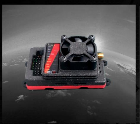
Video transmitter with 1W (+ 30dBm) of RF power and depending on the device it can work in 1.2Ghz, 2.4Ghz or 5.8Ghz with 8 video channels, can be powered from 8-18V, inputs for 2 video cameras with PAL format, 4 auxiliary RC channels (Control only from XLRS transmitters), 1 input Mavlink for to connect the telemetry of the autopilot and a Female-SMA connector to connect an extender together with the omnidirectional antenna.
