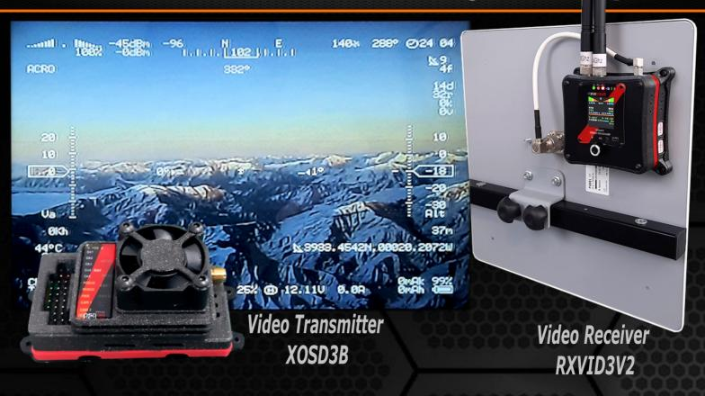
Professional analog video system prepared for all types of FPV applications with 1000mW RF Power in 1.2Ghz, 2.4Ghz or 5.8Ghz to work between 15-40Km (LOS) and with a maximum range of 100km or more depending configuration and antennas.
